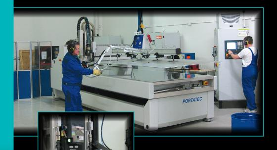
A massive aluminum plate is being loaded on one of YG Acoustics<sup>TM'</sup> CNC machines, custom-made by Portatec in Germany.
